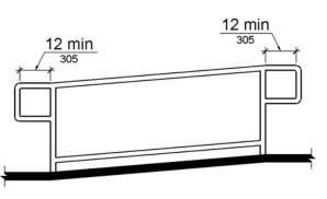
Figure 505.10.1 Top and Bottom Handrail Extension at Ramps
