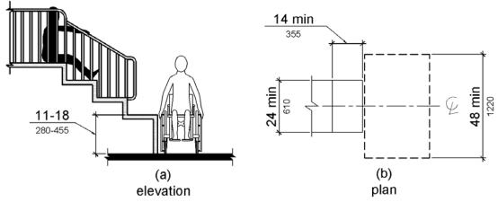
**1008.3.1.4 Transfer Supports.** At least one means of support for transferring shall be provided.
