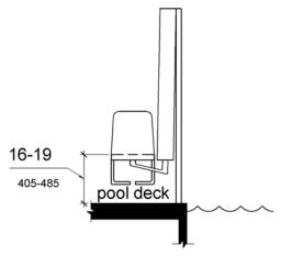
Figure 1009.2.4 Pool Lift Seat Height
