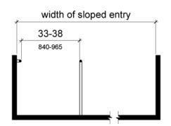
Figure 1009.3.3 Handrails for Sloped Entry
