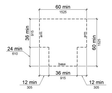
Figure 304.3.2 T-Shaped Turning Space
