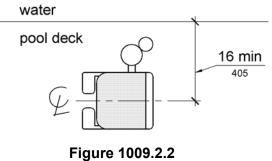
Figure 1009.2.2 Pool Lift Seat Location
