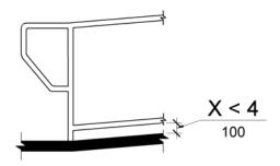
Figure 405.9.2 Curb or Barrier Edge Protection
