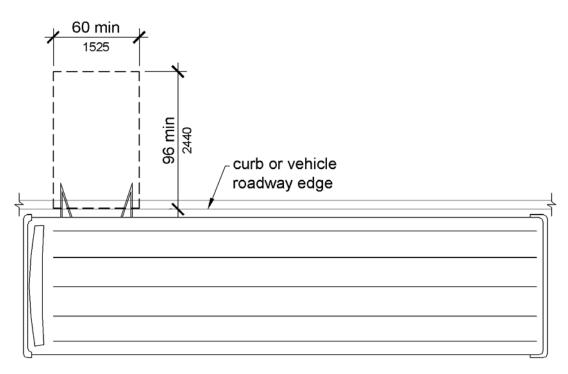
Figure 810.2.2 Dimensions of Bus Boarding and Alighting Areas
