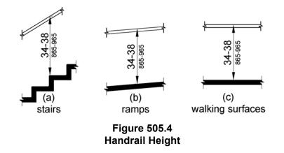
**<sup>505.2</sup> Where Required.** Handrails shall be provided on both sides of stairs and *ramps*. **EXCEPTION:** In *assembly areas*, handrails shall not be required on both sides of aisle *ramps* where a handrail is provided at either side or within the aisle width.
