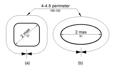
Figure 609.2.2 Grab Bar Non-Circular Cross Section
