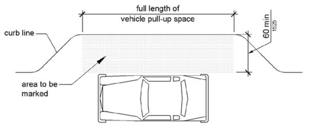
Figure 503.3 Passenger Loading Zone Access Aisle
