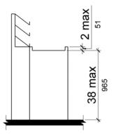
Figure 904.3.2 Check-Out Aisle Counters
