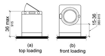
Figure 611.4 Height of Laundry Compartment Opening
