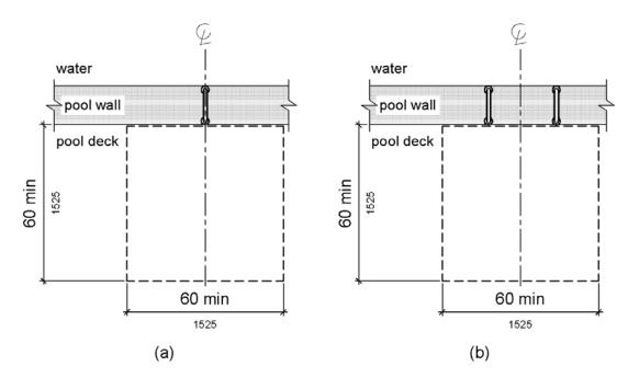
Figure 1009.4.1 Clear Deck Space at Transfer Walls
