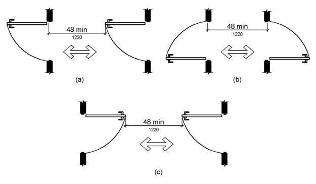
Figure 404.2.6 Doors in Series and Gates in Series
