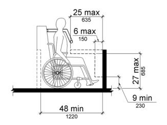
Figure 1002.4.4.3 Protrusions in Wheelchair Spaces in Amusement Rides
