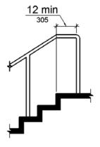
Figure 505.10.2 Top Handrail Extension at Stairs
