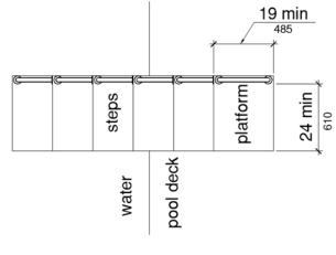
Figure 1009.5.1 Size of Transfer Platform
