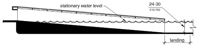
Figure 1009.3.2 Sloped Entry Submerged Depth
