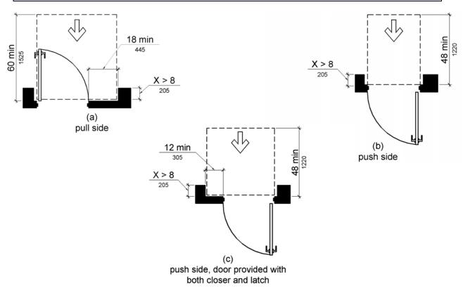
Figure 404.2.4.3 Maneuvering Clearances at Recessed Doors and Gates
