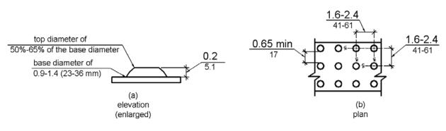
Figure 705.1 Size and Spacing of Truncated Domes
