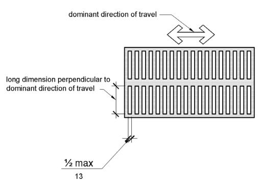
Figure 302.3 Elongated Openings in Floor or Ground Surfaces
