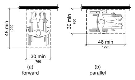
Figure 305.5 Position of Clear Floor or Ground Space
