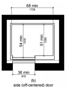
Figure 407.4.1 Elevator Car Dimensions
