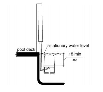
Figure 1009.2.8 Pool Lift Submerged Depth
