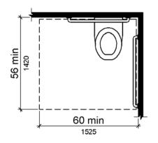
Figure 604.3.1 Size of Clearance at Water Closets
