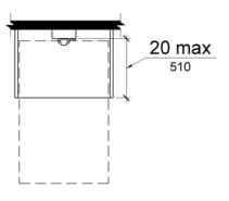
Figure 704.2.1.2 Forward Approach to Telephone
