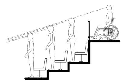
Figure 802.2.2.2 Lines of Sight Between the Heads of Standing Spectators
