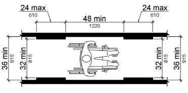
Figure 403.5.1 Clear Width of an Accessible Route
