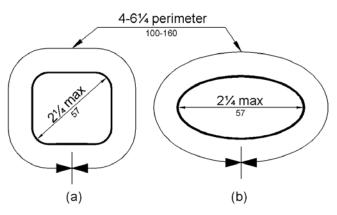
Figure 505.7.2 Handrail Non-Circular Cross Section
