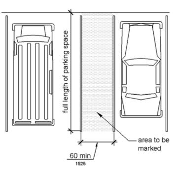
Figure 502.3 Parking Space Access Aisle
