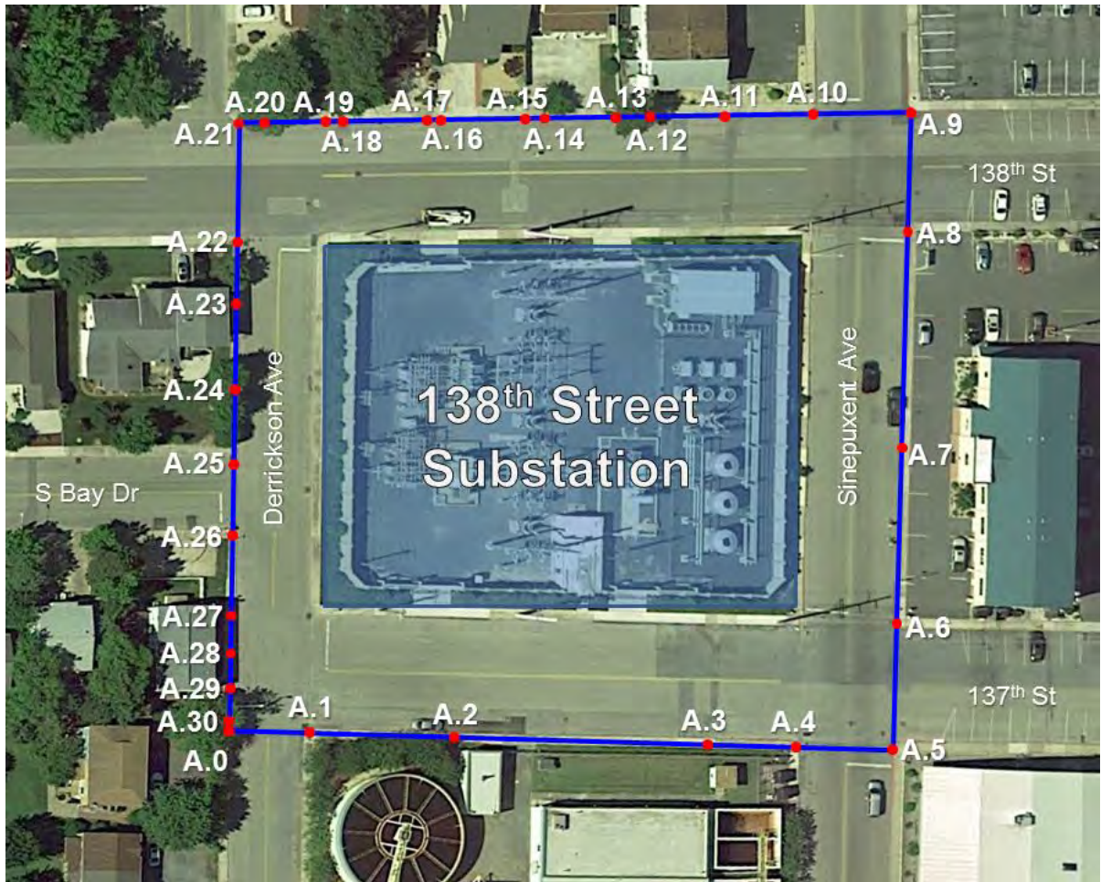
Figure 1. Aerial view of the 138th Street Substation between Derrickson Avenue and Sinepuxent Avenue showing the measurement path along the outer perimeter across the street from the substation.
